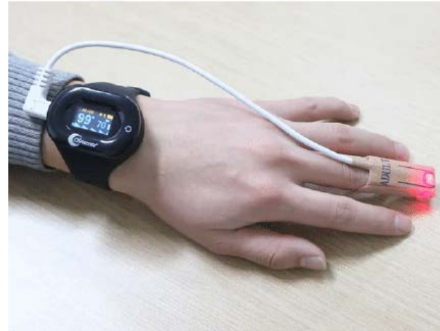
Wrist watch based 24/7 fingertip pulse oxymeter
